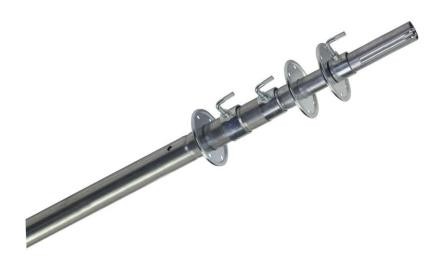
Three galvanized pieces of mechanical tubing; outside section 1.75" OD - 18 gauge; second section 1.50" -18 gauge OD; inside section 1.25" OD- 16 gauge.
